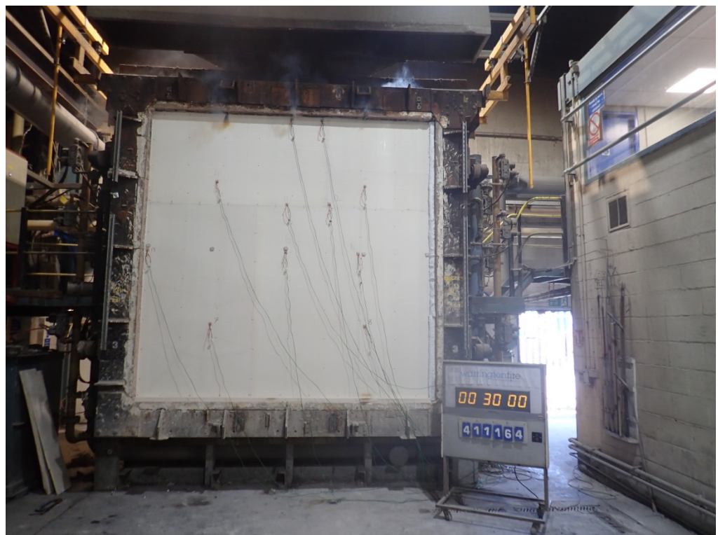
The unexposed face of the test specimen after 30 minutes of testing
