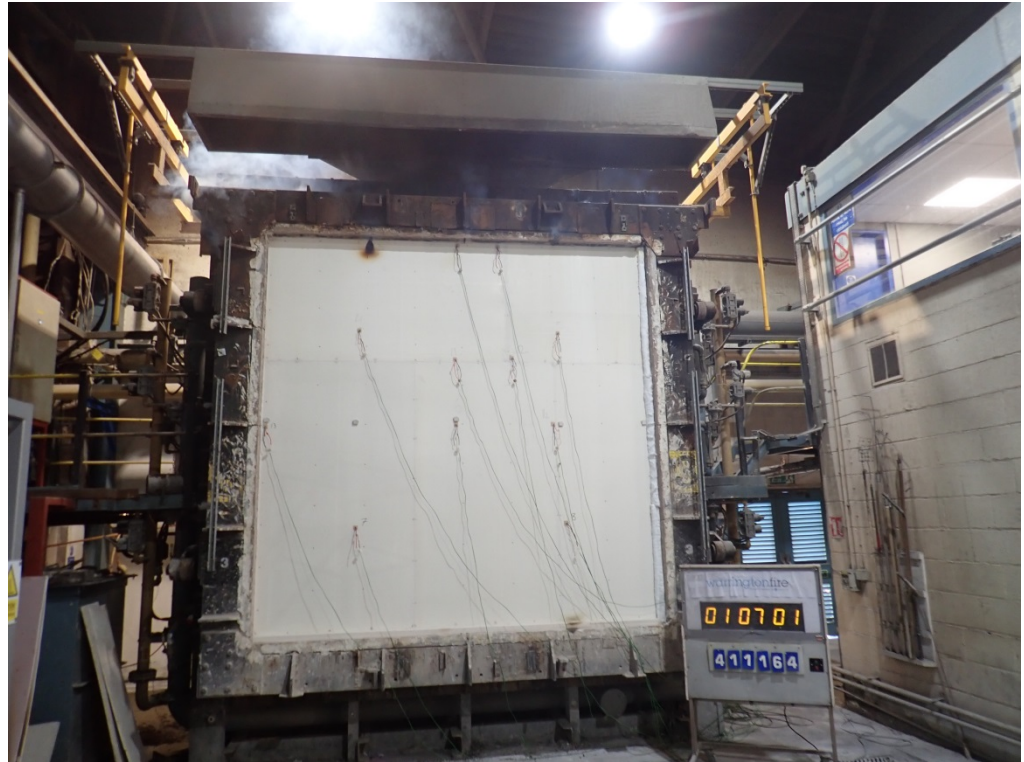
The unexposed face of the test specimen after 67 minutes of testing
