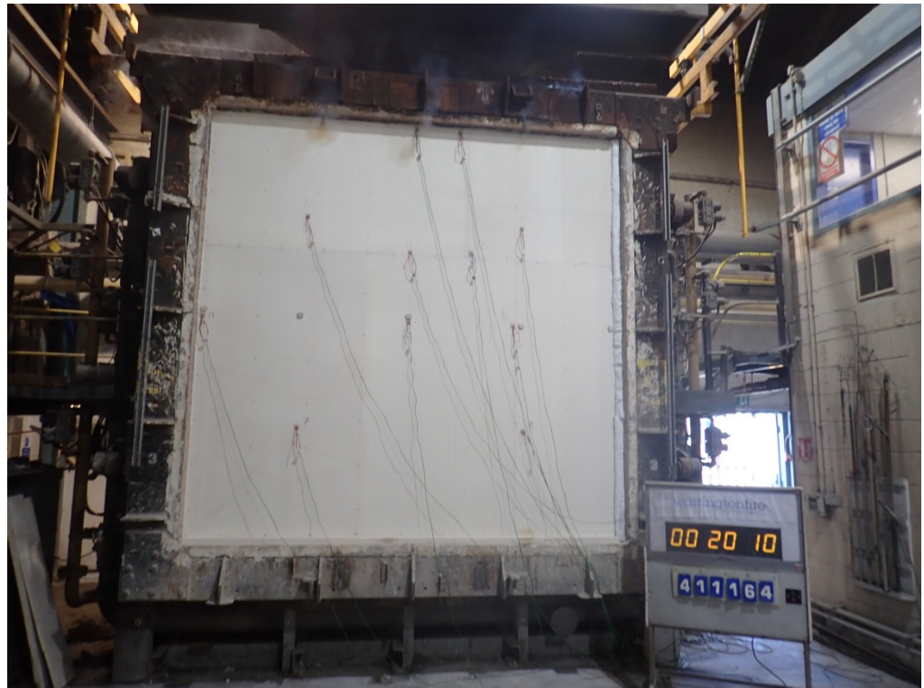
The unexposed face of the test specimen after 20 minutes of testing
