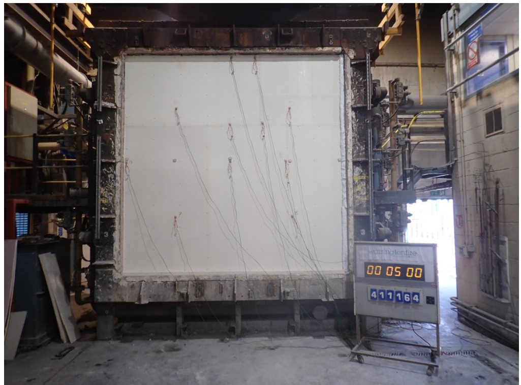
The unexposed face of the test specimen after 5 minutes of testing
